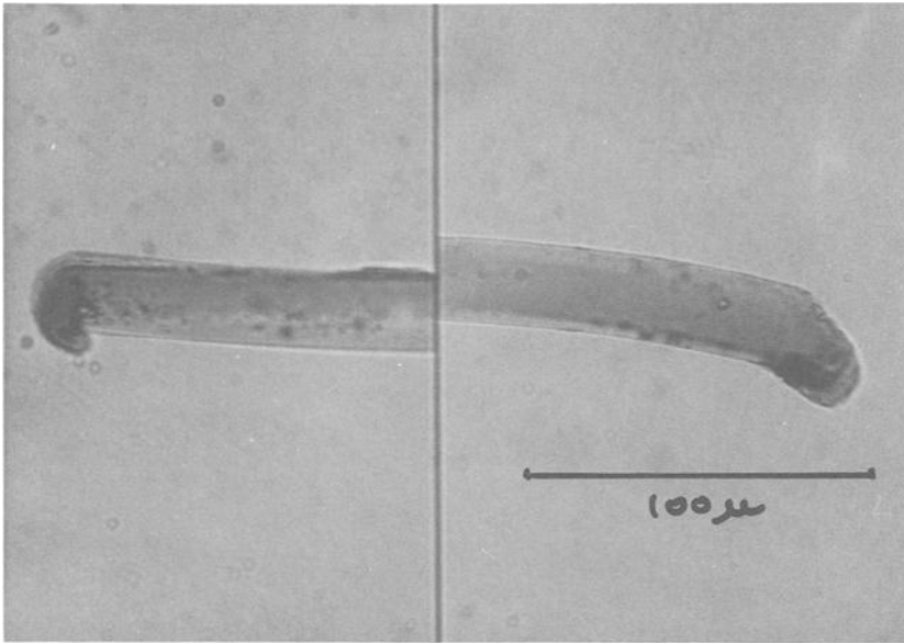
FIG. 2—Comparison photomicrograph of known fibers from the upholstery in the suspect's vehicle (left) and fibers isolated from the victim's underpants (right). (Approximate magnification \times 450 ).
